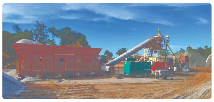
Concrete Batching/Mixing Plant Turbo Pan Mixer / Planetary Pan Mixer / Twin Shaft Mixer (Output : 20 to 120 Cum./hr.)
