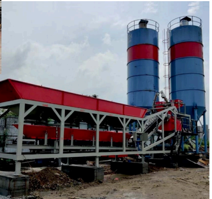
Compact Concrete Batching/Mixing Plant Turbo Pan Mixer / Planetary Mixer / Twin Shaft Mixer (Output : 20 to 60 Cum./hr.)
